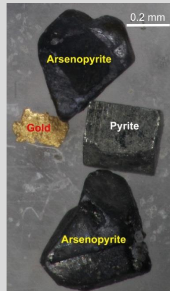
Figure C26. Unoxidised sulphide minerals in >12,000-year-old sediments from Macraes mine.
