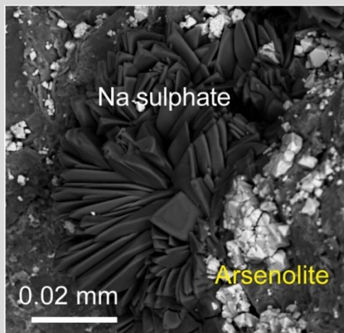
Figure C12. Scanning electron microscope image of evaporative minerals on leached arsenopyrite.
