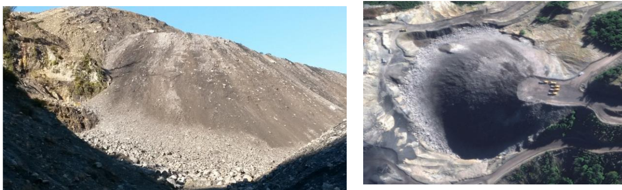
Figure 29. Grain-size segregation at PAF coal mines, New Zealand.
