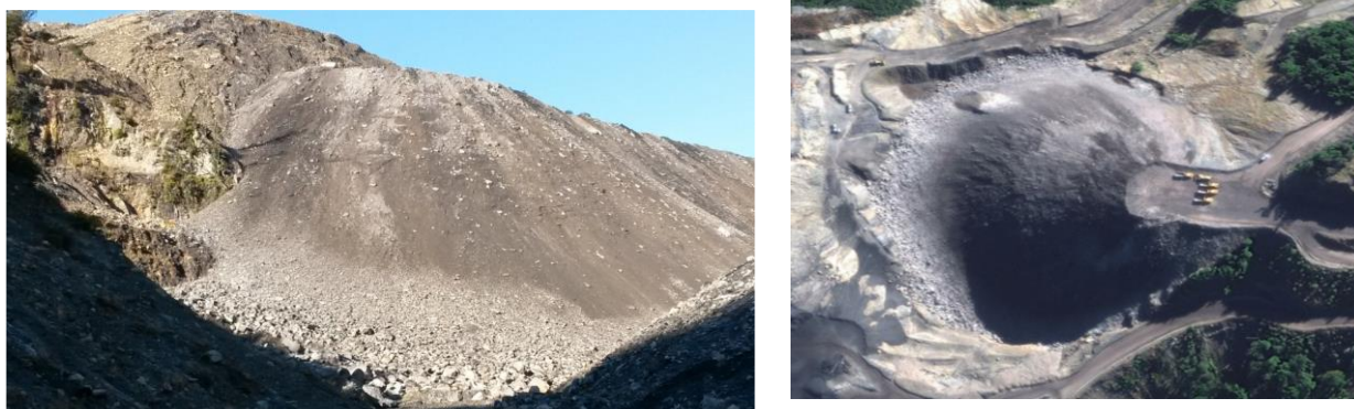
Figure 32. Grain-size segregation at PAF coal mines, New Zealand.
