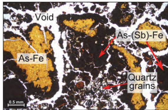
**Figure 7.** Microphotograph of sample B-2, taken under plane-polarized light (PPL), showing subrounded quartz grains and two distinctive secondary mineral phases.
