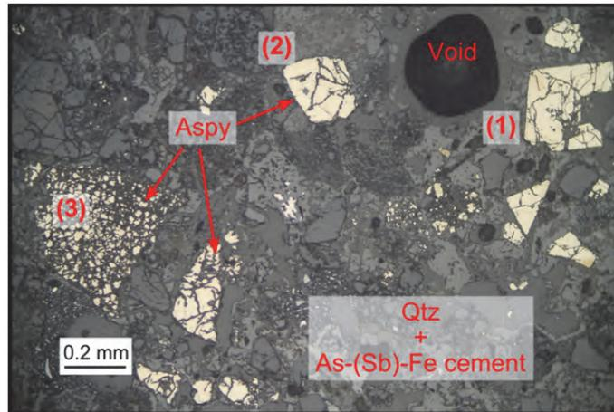
**Figure 4.** Reflected light microscope (REF) image of sample B-1 showing arsenopyrite grains at different stages of decomposition.
