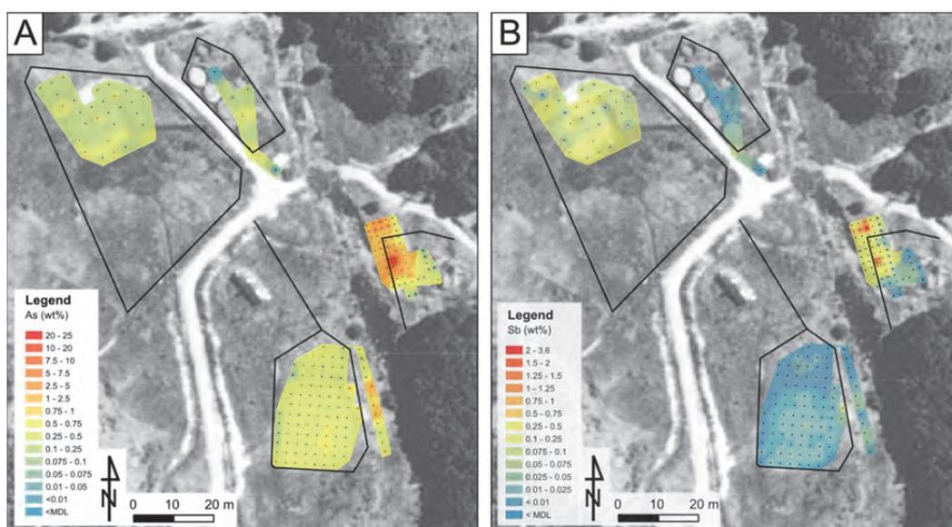
**Figure 3.** Maps showing As (A) and Sb (B) contents distribution (in wt%) at the Big River Mine's processing site. The maps were created using corrected results of the FPXRF analyses. Solid lines show existing fences.
