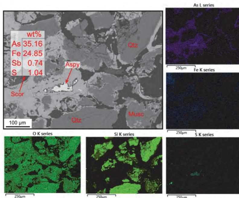
**Figure 5.** BSE image showing a decomposing arsenopyrite grain, with corresponding elemental (As, Fe, S, Si, O) maps. Results of selected EDS spot analysis are also shown.
