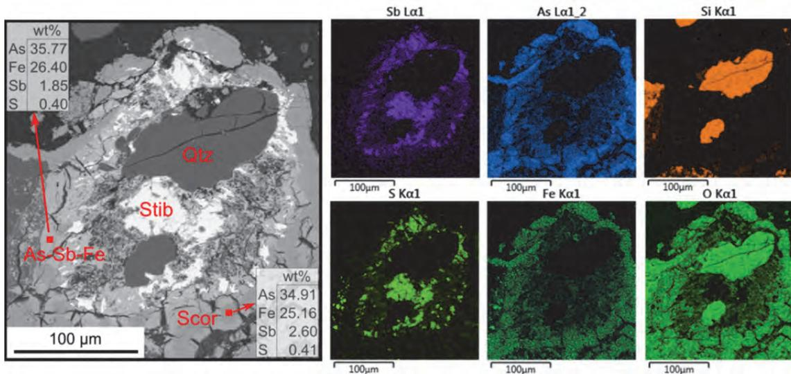
**Figure 6.** BSE image showing a decomposing stibnite grain, with corresponding elemental (Sb, S, As, Fe, Si, O) maps. Results of selected EDS spot analyses are also shown.
