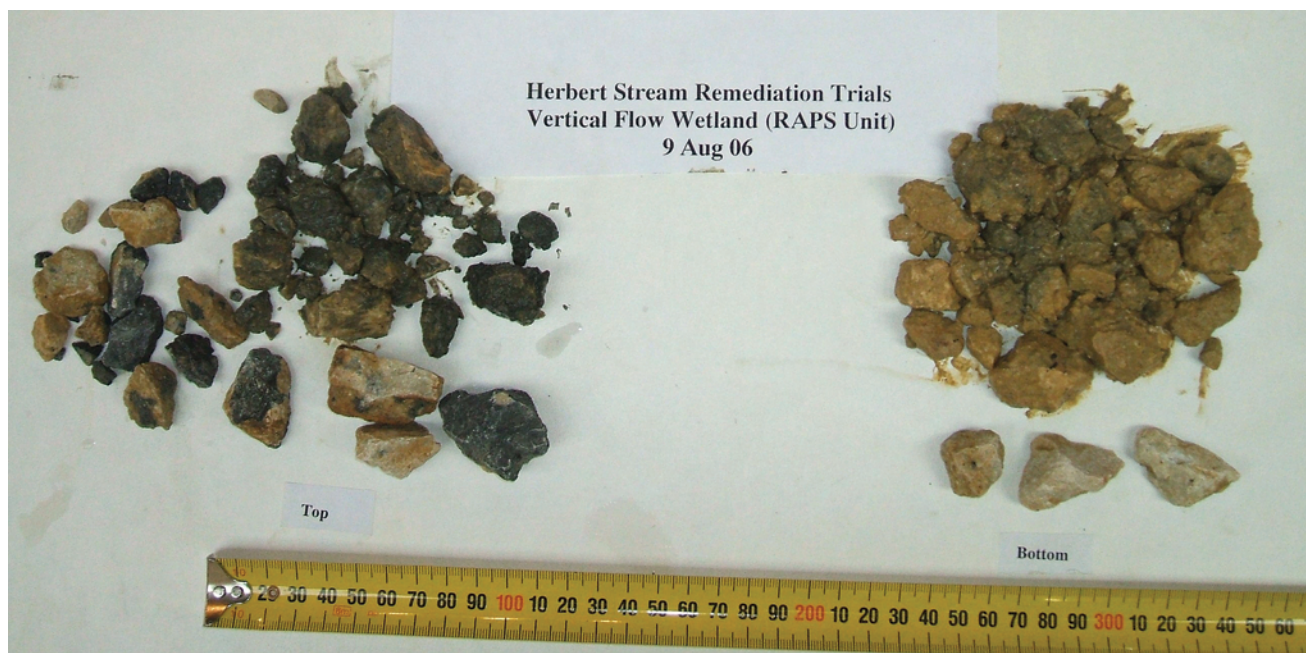
Fig. 10 Limestone from the reducing and alkalinity producing system post-pilot trials showing extent of armouring by Fe monosulfides and hydroxides. Top, Bottom designates location in the system. Rocks along the top of the photo are unwashed; rocks along the bottom were rinsed briefly. Unwashed rocks are associated with black deposits at the top of the limestone layer and brownish yellow deposits at the base. Washed rocks show minimal covering with reddish precipitates in both layers.
