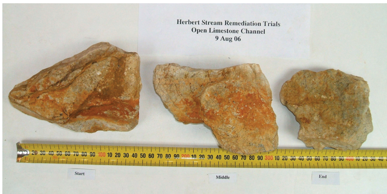
Fig. 11 Limestone from the open limestone channel post-pilot trials showing extent of armouring by Fe hydroxides. Start, Middle, End designates location in the system. The rocks exhibit a marked decrease in percent covering with precipitates and a change in colour from reddish to yellowish down the channel.
